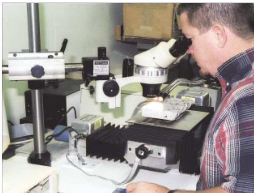
With the sample mounted on a moving table, the petrographer is able to count each air bubble—entrained and entrapped.
