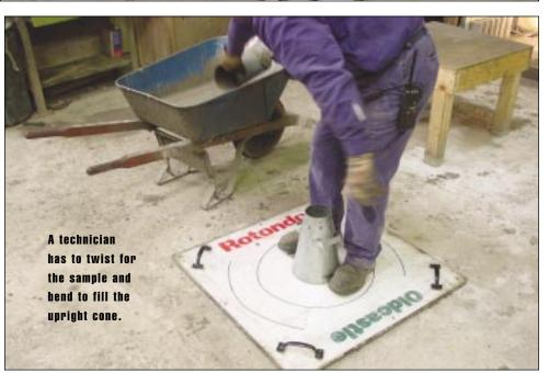
Although no standards have been established, testing slump flow is an everyday reality.
