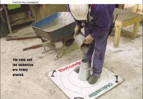
the cone can be maneuvered without the producer's feet coming into play. Most producers using the inverted method agree the weight of the concrete in the cone holds it downward so that a person does not have to stand on it. With the cone inverted, a Plexiglas "flow board" can be elevated so there is no need to bend over. And if your feet are not tied down, you are free to move around instead of stretching and twisting for the next scoop of concrete.
