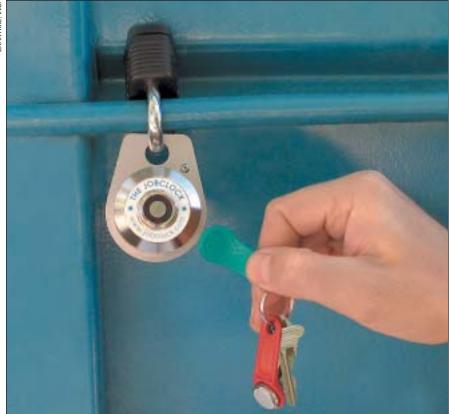
Touching color-coded key tabs to the weatherproof, construction-grade clock logs start and stop times.
